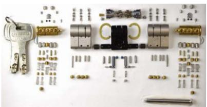
A modern cylinder disassembled demonstrating the amazing range of technological perceived weaknesses. Does bumping for instance solutions embedded within. There are some six box framed similar variations in the ever occur to a lock in situ, are there any instances MLA HQ Training Room.
