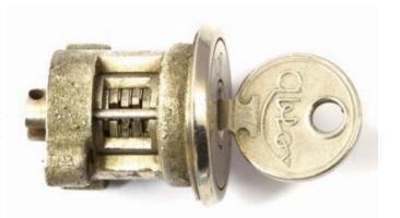
An early Abloy factory cutaway cylinder showing the rotating discs with the side bar resting on their peripheries, the key rotates to align slots in the discs to align with the side bar allowing it to drop into the slots thereby providing the drive on further rotation.
